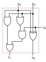
✓ Implement  $c_1$  using ONLY 2-to-1 MUXs (AND, OR, NOT, XOR gates are not allowed). (12 pts)  $c_1(x_0, y_0, c_0) = x_0y_0 + x_0c_0 + y_0c_0$
